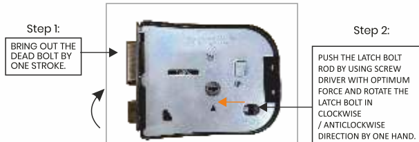
Image 1 :- Procedure for changing Latch bolt orientation
